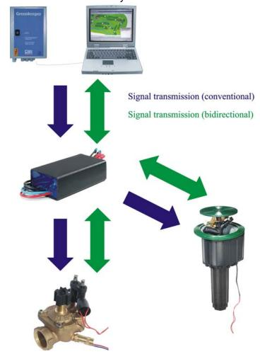
The Greenkeeper Control system compares the planned and actual value. In case of divergence immediately a dialog field with ERORR STATUS appears with the replied error.
