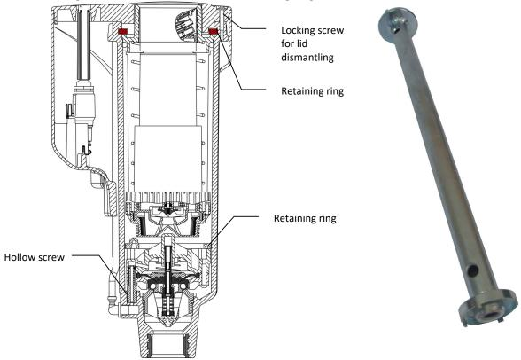
☆ Pull sprinkler insert out of the housing
