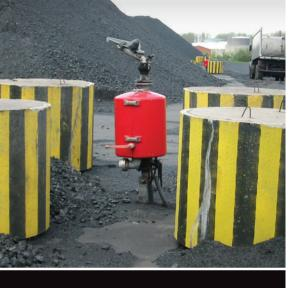
Sprinklers can operate in harsh outdoor environments and conditions to prevent dust from blowing around.
