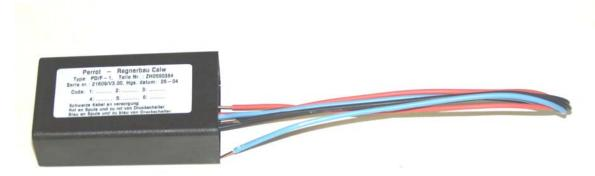
The feedback decoder communicates with the control centre in both directions. It can receive information and implement the associated instructions. On the other hand it sends information over the actual condition of the station back to the
