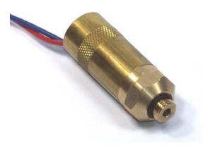
The pressure sensor gives the information to the decoder, whether there is enough pressure at the sprinkler. The pressure threshold is adjusted to 2,5 bar. This is the minimum required pressure for the reliable operation of the sprinkler.
