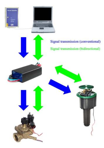
In addition to the information <u>if water flows or no</u>t, the <u>feedback</u> decoder can report further state diagnostics to the central office:
