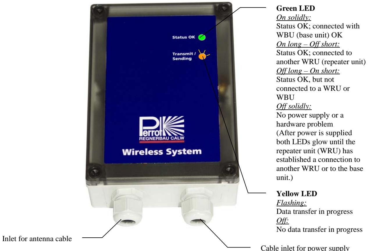
Power can be supplied to the WRU via a power supply unit (see 2.2.1) or decoder line adapter (2.2.2), as preferred.
